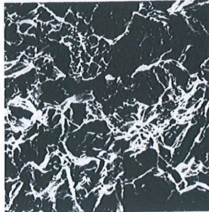
700:1 electromicroscopic image of the hardened layer of a tooth after breakage. The fracture surface shows the distribution of intergranular fracture structure and transcrystalline fracture honeycomb structure.
