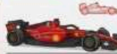
2022 FERRARI F1-75 GROUND EFFECT RETURN, WIDE SIDEPODS
